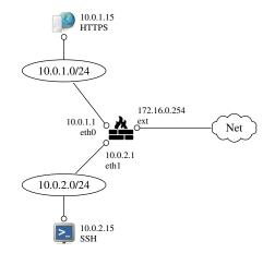
Figure 1: A case study of a firewall with three interfaces.
